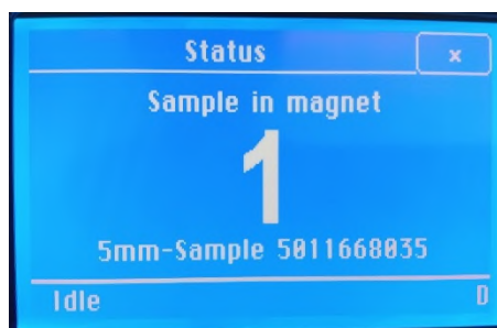
Figure 12: SampleJet interface in automation mode and when sample 1 is present in the magnet
