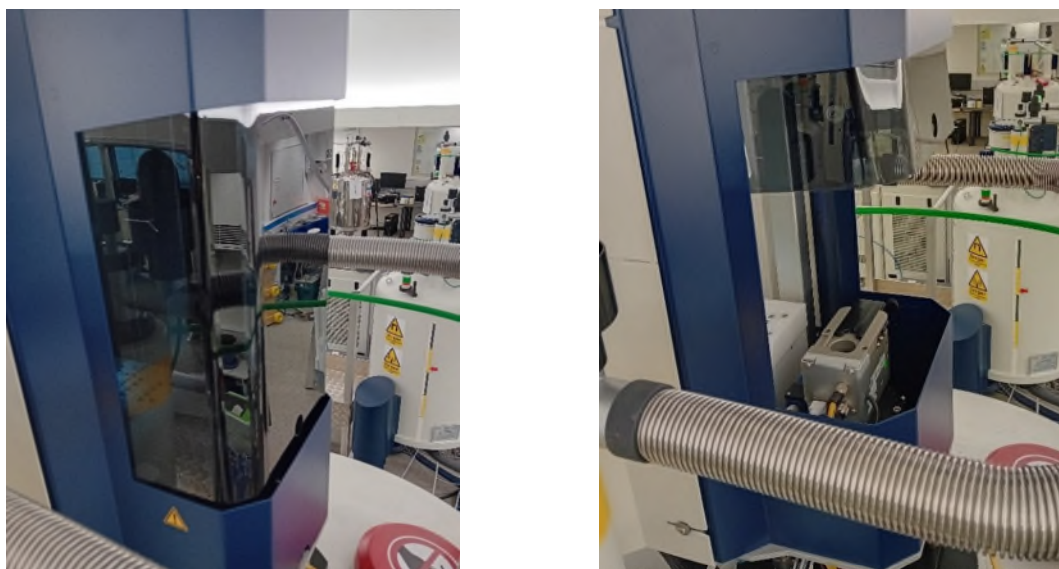
Figure 10: (left) Black plastic cover in its default position and (right) raised and secured in place to gain access to the magnet bore.
