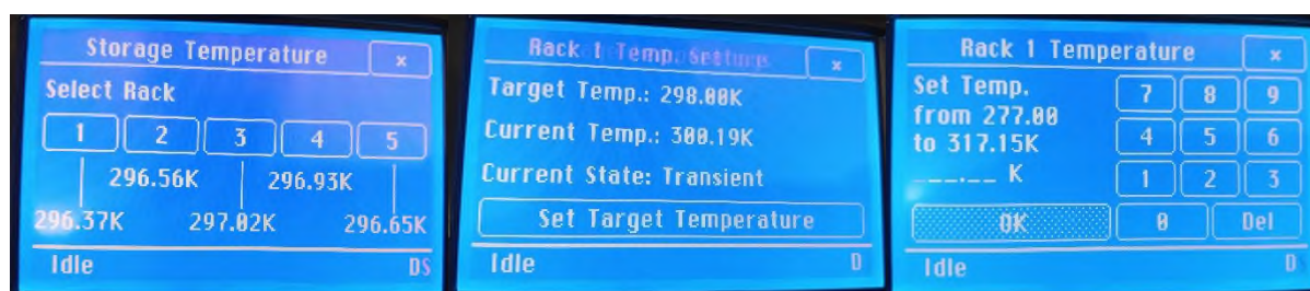
Figure 14: SampleJet interface when adjusting the storage temperature. (left) Overview of the storage temperature for all racks, (middle) rack 1 temperature and (right) setting of the rack 1 temperature.
